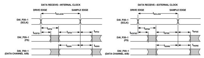
NOTE: EITHER THE RISING EDGE OR FALLING EDGE OF SCLK (EXTERNAL) OR SCLK (INTERNAL) CAN BE USED AS THE ACTIVE SAMPLING EDGE.
