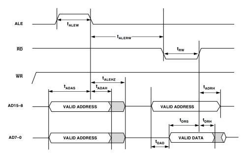
Figure 17. 8-Bit Memory Read Cycle
