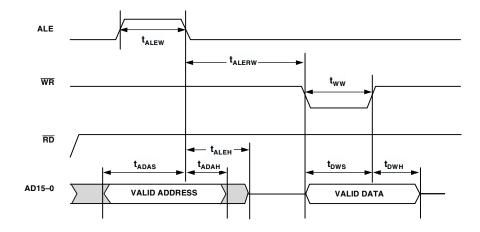
Figure 20. 16-Bit Memory Write Cycle
