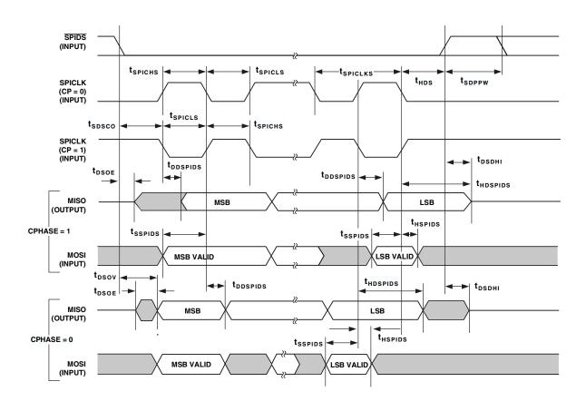
Figure 26. SPI Protocol—Slave
