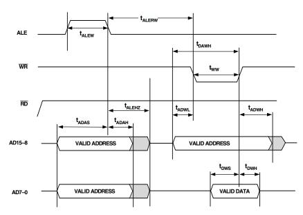
Figure 19. 8-Bit Memory Write Cycle
