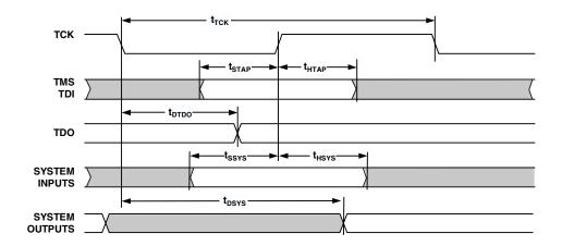
Figure 27. JTAG Test Access Port and Emulation
