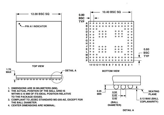
Figure 35. 136-Ball Mini-BGA [CSP\_BGA] (BC-136-3)
