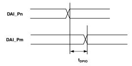
Figure 14. DAI Pin-to-Pin Direct Routing
