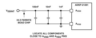
Figure 4. Analog Power Filter Circuit
