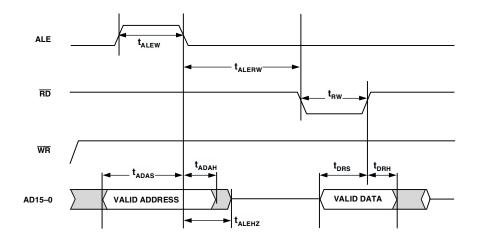
Figure 18. 16-Bit Memory Read Cycle
