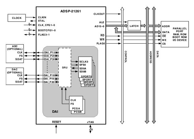
Figure 2. ADSP-21261 System Sample Configuration
