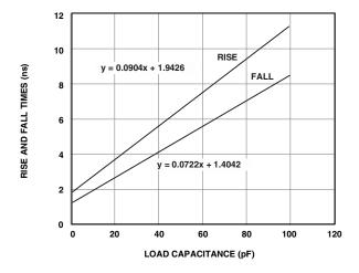
Figure 31. Typical Output Rise/Fall Time (20% to 80%, V<sub>DDEXT</sub> = Max)
