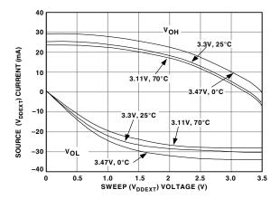
Figure 28. ADSP-21261 Typical Drive
