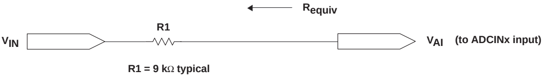
Figure 47. Typical ADC Input Pin Circuit
