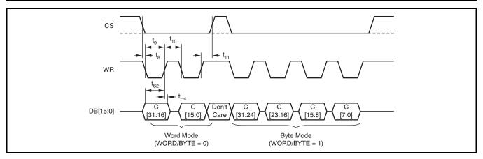
Figure 3. Parallel Write Access Timing Diagram
