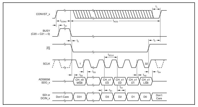
Figure 1. Serial Operation Timing Diagram (All Three SDOs Active)
