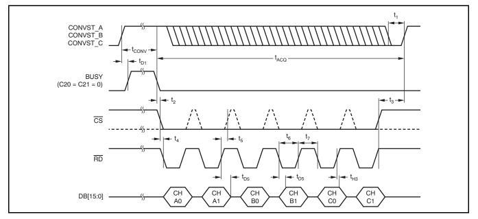
Figure 2. Parallel Read Access Timing Diagram
