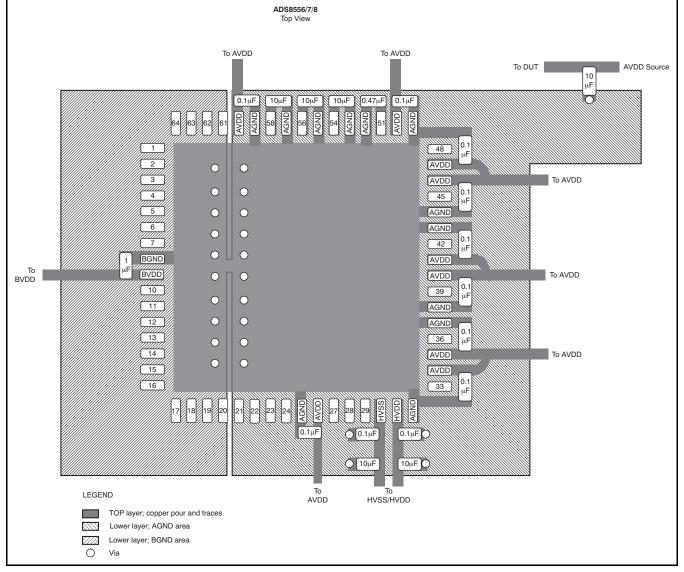
(1) All  $0.1\mu F$ ,  $0.47\mu F$ , and  $1\mu F$  capacitors should be placed as close to the ADS8556/7/8 as possible.
