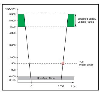
Figure 40. POR: Relevant Voltage Levels
