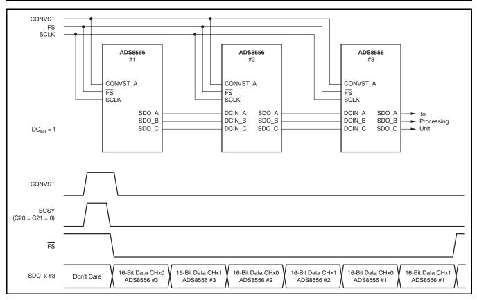
Figure 39. Example of Daisy-Chaining Three ADS8556s
