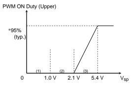
\*: The maximum ON duty is  $T_{ON} = 95\%$  (typ.) when  $V_{SP} = 5.4 \text{ V}$  (typ.). Example: If  $f_{OSC} = 5 \text{ MHz}$ , then ON time = 48  $\mu s$  (typ.) ( $f_{C} = 19.8 \text{ kHz}$ ) If  $f_{OSC} = 4 \text{ MHz}$ , then ON time = 60  $\mu s$  (typ.) ( $f_{C} = 15.9 \text{ kHz}$ )
