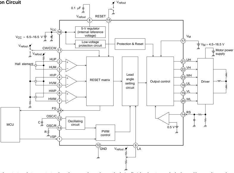
Any short circuit between the outputs, or between output and supply or ground, may damage the device. Peripheral parts may also be damaged by overvoltage and overcurrent. Design the output lines,  $V_{CC}$ ,  $V_{M}$  and GND lines so that short circuits do not occur.
