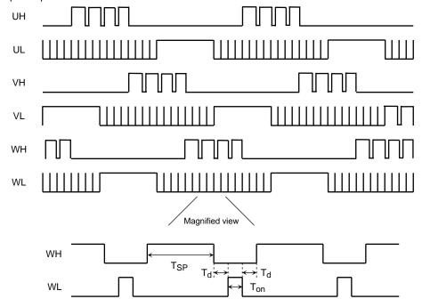
$T_{SP}$ : Variable depending on the  $V_{SP}$  (the figure above being applicable when  $V_{SP} = 5.4 \text{ V}$  (typ.));  $T_{ON} = 18/f_{OSC}$ ;  $T_{CS} = 18/f_{OSC}$
