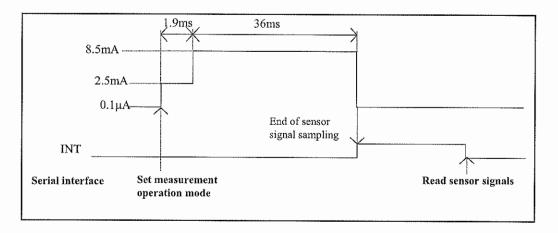
Note) While the INT pin is held "H", sensor signal sampling does not start even when measurement operation mode is set. Before setting measurement operation mode, check that the INT pin is "L", or perform a dummy sensor signal read to drive the INT pin "L".
