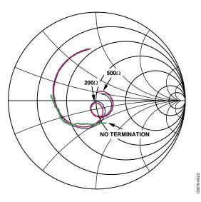
Figure 23. Smith Chart of LOIP Port  $S_{11}$  (LOIN Pin AC-Coupled to Ground). Curves with Balun and External Termination Resistors Also Shown ( $T_A = 25^{\circ}C$ )
