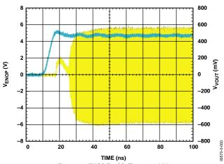
Figure 49. ENOP Enable Time, 900 MHz
