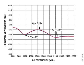
Figure 13. Sideband Suppression vs.  $F_{LO}$  ( $F_{BB} = 1$  MHz, I and Q Inputs Driven in Quadrature at 1.2 V p-p Differential,  $T_A = 25$ °C)
