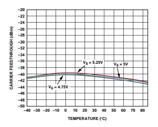
Figure 12. Carrier Feedthrough vs. Temperature ( $F_{LO} = 2140 \, \text{MHz}$ ,  $F_{BB} = 1 \, \text{MHz}$ , I and Q Inputs Driven in Quadrature at 1.2 V p-p Differential,  $T_A = 25 \, ^{\circ}\text{C}$ )
