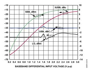
Figure 19. Third Order Distortion (3USB), Carrier Feedthrough, Sideband Suppression, and SSB  $P_{OUT}$  vs. Baseband Differential Input Level ( $F_{LO} = 900$  MHz,  $F_{BB} = 1$  MHz, I and Q Inputs Driven in Quadrature,  $T_A = 25^{\circ}$ C)
