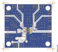
Figure 66. Layout of Evaluation Board, Top Layer
