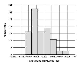
Figure 34. I and Q Inputs Quadrature Phase Imbalance Distribution ( $F_{LO} = 2140$  MHz,  $F_{BB} = 1$  MHz, I and Q Inputs Driven in Quadrature at 1.2 V p-p Differential,  $T_A = 25$ °C)
