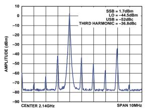
Figure 53. AD8349 Single Sideband Spectrum at 2140 MHz
