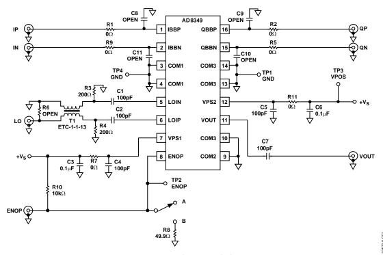
Figure 68. Evaluation Board Schematic
