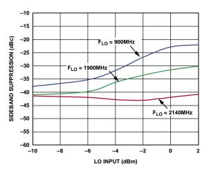
Figure 33. Sideband Suppression vs. LO Input Power ( $F_{BB} = 1 \text{ MHz}$ , I and Q Inputs Driven in Quadrature at 1.2 V p-p Differential,  $T_A = 25 \,^{\circ}\text{C}$ )
