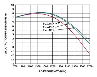
Figure 10. SSB Output 1 dB Compression Point (OP1dB) vs.  $F_{LO}$  ( $F_{BB}$  = 1 MHz, I and Q Inputs Driven in Quadrature,  $T_A$  = 25°C)
