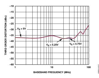
Figure 17. Third Order Distortion vs.  $F_{BB}$  ( $F_{LO}$  = 2140 MHz, I and Q Inputs Driven in Quadrature at 1.2 V p-p Differential,  $T_A$  = 25°C)
