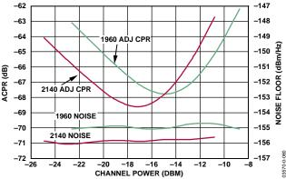
Figure 59. Single-Carrier WCDMA ACPR and Noise Floor (dBm/Hz) at 30 MHz Carrier Offset vs. Channel Power at 1960 MHz and 2140 MHz (Test Model 1 with 64 Active Channels)
