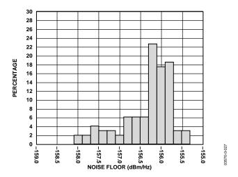
Figure 27. 20 MHz Offset Noise Floor Distribution at  $F_{LO}$  = 2140 MHz (BB Inputs at a Bias of 400 mV with no AC signal,  $T_A$  = 25°C)
