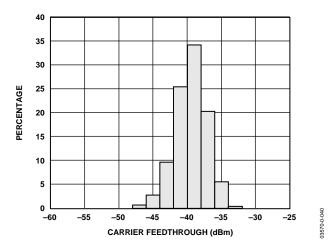
Figure 38. Carrier Feedthrough Distribution at  $F_{LO} = 1900$  MHz ( $F_{BB} = 1$  MHz, I and Q Inputs Driven in Quadrature at 1.2 Vp-p,  $T_A = 25$ °C)
