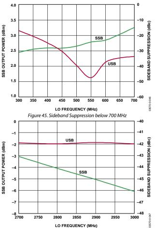
Figure 46. Sideband Suppression above 2700 MHz
