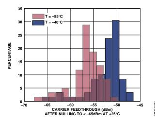
Figure 40. Carrier Feedthrough Distribution at Temperature Extremes, After Carrier Feedthrough Nulled to < - 65 dBm at  $T_A = 25^{\circ}$ C. ( $F_{LO} = 2140$  MHz, I and Q Inputs at a bias of 400 mV)
