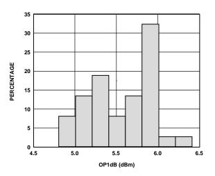
Figure 36. OP1dB Distribution. ( $F_{LO}=2140$  MHz,  $F_{BB}=1$  MHz, I and Q Inputs Driven in Quadrature,  $T_A=25^{\circ}C$ )
