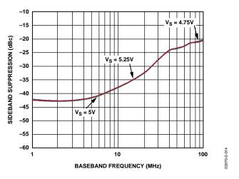
Figure 14. Sideband Suppression vs.  $F_{BB}$  ( $F_{LO}$  = 2140 MHz, I and Q Inputs Driven in Quadrature at 1.2 V p-p Differential,  $T_A$  = 25°C)
