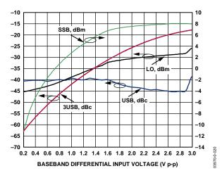
Figure 20. Third Order Distortion (3USB), Carrier Feedthrough, Sideband Suppression, and SSB  $P_{OUT}$  vs. Baseband Differential Input Level ( $F_{LO} = 1900 \text{ MHz}$ ,  $F_{BB} = 1 \text{ MHz}$ , I and Q Inputs Driven in Quadrature,  $T_A = 25^{\circ}\text{C}$ )
