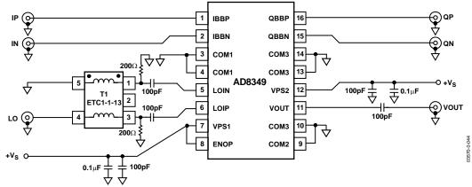
Figure 43. Basic Connections
