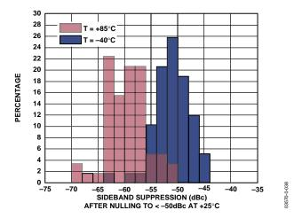
Figure 41. Sideband Suppression Distribution at Temperature Extremes, After Sideband Suppression Nulled to < -50 dBc at  $T_A = 25$ °C. ( $F_{LO} = 2140$  MHz,  $F_{BB} = 1$  MHz, I and Q Inputs biased at 0.4 V)
