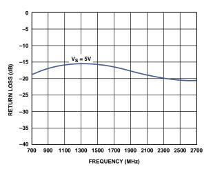
Figure 24. Return Loss  $S_{22}$  of  $V_{OUT}$  Output ( $T_A = 25$ °C)
