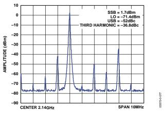
Figure 55. AD8349 Single Sideband Spectrum at 2140 MHz after LO Nulling
