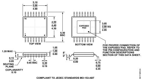
Figure 70. 16-Lead Thin Shrink Small Outline with Exposed Pad [TSSOP\_EP] (RE-16-2) Dimensions shown in millimeters
