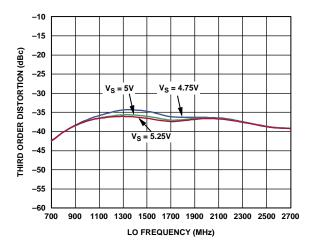
Figure 16. Third Order Distortion vs.  $F_{LO}$  ( $F_{BB} = 1$  MHz, I and Q Inputs Driven in Quadrature at 1.2 V p-p Differential,  $T_A = 25$ °C)
