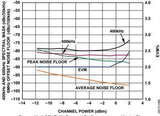
Figure 63. 8-PSK EVM, Spectral Performance, and Noise Floor vs. Channel Power (Frequency = 885 MHz)
