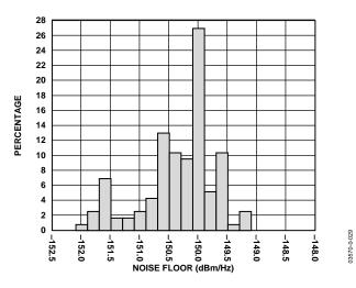
Figure 29. 20 MHz Offset Noise Floor Distribution at  $F_{LO}$  = 1960 MHz ( $F_{BB}$  = 1 MHz, I and Q Inputs Driven in Quadrature at 1.2 V p-p,  $T_A$  = 25°C)
