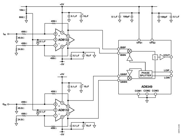
Figure 44. Single-Ended IQ Drive Circuit
