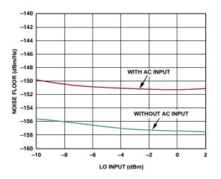
Figure 31. 20 MHz Offset Noise Floor vs. LO Input Power  $(F_{LO}=2140$  MHz,  $T_A=25$  °C)
