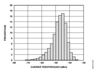
Figure 37. Carrier Feedthrough Distribution at  $F_{LO}=900$  MHZ ( $F_{BB}=1$  MHz, I and Q Inputs Driven in Quadrature at 1.2 V p-p,  $T_A=25$ °C)
