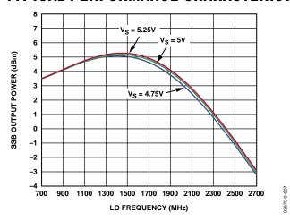
Figure 7. Single Sideband (SSB) Output Power ( $P_{OUT}$ ) vs. LO Frequency ( $F_{LO}$ ) (I and Q Inputs Driven in Quadrature at Baseband Frequency ( $F_{BB}$ ) = 1 MHz, I and Q Inputs at 1.2 V p-p Differential,  $T_A$  = 25°C)
