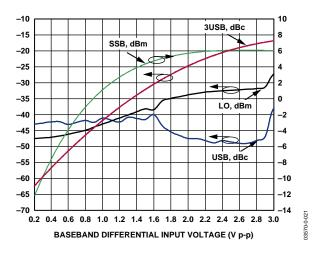
Figure 21. Third Order Distortion (3USB), Carrier Feedthrough, Sideband Suppression, and SSB  $P_{OUT}$  vs. Baseband Differential Input Level ( $F_{LO} = 2140$  MHz,  $F_{BB} = 1$  MHz, I and Q Inputs Driven in Quadrature,  $T_A = 25^{\circ}$ C)
