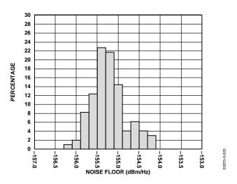
Figure 25. 20 MHz Offset Noise Floor Distribution at  $F_{LO} = 900$  MHz (BB Inputs at a Bias of 400 mV with no AC signal,  $T_A = 25$ °C)
