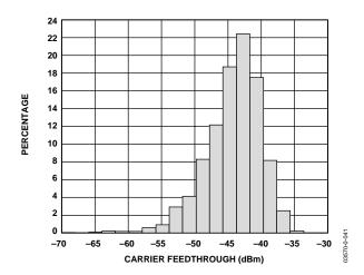
Figure 39. Carrier Feedthrough Distribution at  $F_{LO}=2140$  MHz ( $F_{BB}=1$  MHz, I and Q Inputs Driven in Quadrature at 1.2 V p-p,  $T_A=25$ °C)
