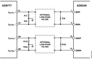
Figure 51. Basic AD9777 to AD8349 Interface
