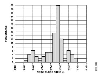
Figure 26. 20 MHz Offset Noise Floor Distribution at  $F_{LO} = 1900$  MHz (BB Inputs at a Bias of 400 mV with no AC signal,  $T_A = 25$ °C)
