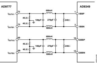
Figure 57. Single-Carrier WCDMA Application Circuit (DAC-Modulator Interconnect)
