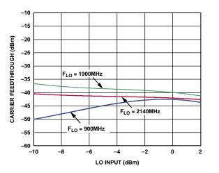
Figure 32. Carrier Feedthrough vs. LO Input Power ( $F_{BB} = 1 \text{ MHz}$ , I and Q Inputs Driven in Quadrature at 1.2 V p-p Differential,  $T_A = 25^{\circ}\text{C}$ )
