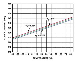
Figure 22. Power Supply Current vs. Temperature
