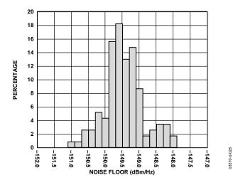
Figure 28. 20 MHz Offset Noise Floor Distribution at  $F_{LO}=940$  MHz ( $F_{BB}=1$  MHz, I and Q Inputs Driven in Quadrature at 1.2 V p-p,  $T_A=25^{\circ}$ C)
