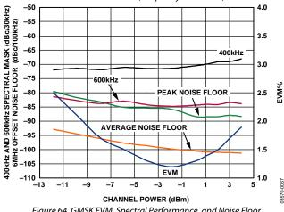
Figure 64. GMSK EVM, Spectral Performance, and Noise Floor vs. Channel Power (Frequency = 1960 MHz)
