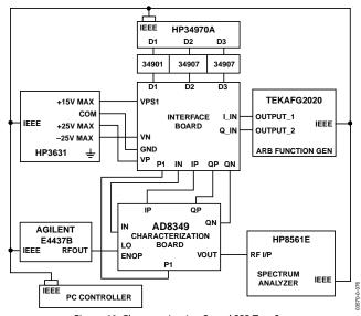
Figure 69. Characterization Board SSB Test Setup
