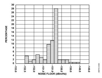
Figure 30. 20 MHz Offset Noise Floor Distribution at  $F_{LO} = 2140$  MHz ( $F_{BB} = 1$  MHz, I and Q Inputs Driven in Quadrature at 1.2 V p-p,  $T_A = 25^{\circ}$ C)
