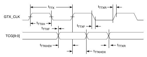
Figure 12. TBI Transmit AC Timing Diagram
