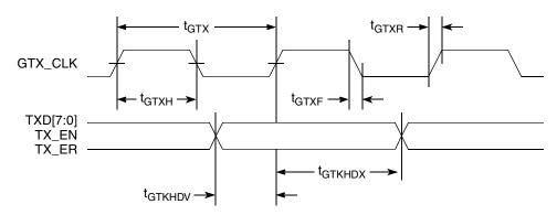
Figure 7. GMII Transmit AC Timing Diagram
