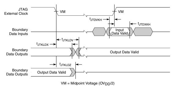
Figure 34. Boundary-Scan Timing Diagram
