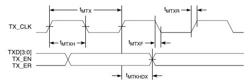
Figure 10. MII Transmit AC Timing Diagram
