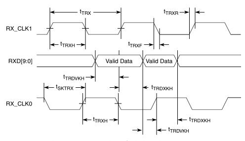
Figure 13. TBI Receive AC Timing Diagram
