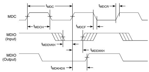
Figure 15. MII Management Interface Timing Diagram
