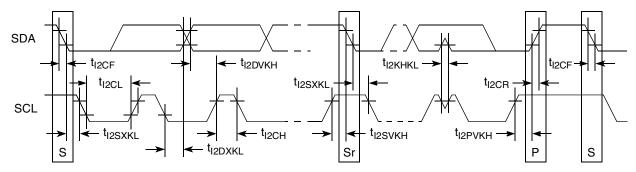
Figure 37. I<sup>2</sup>C Bus AC Timing Diagram
