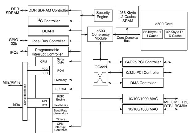
Figure 1. MPC8541E Block Diagram
