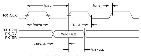
Figure 11. MII Receive AC Timing Diagram
