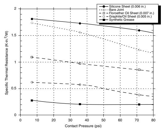
Figure 45. Thermal Performance of Select Thermal Interface Materials
