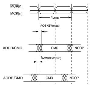
Figure 4. Timing Diagram for  $t_{\text{AOSKEW}}$  Measurement
