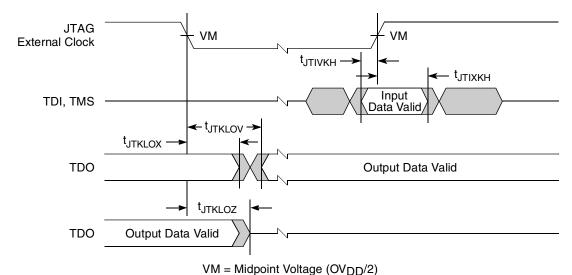
Figure 35. Test Access Port Timing Diagram
