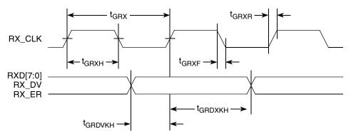
Figure 9. GMII Receive AC Timing Diagram
