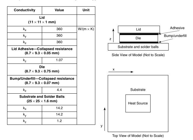
Figure 43. MPC8541E Thermal Model
