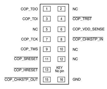
Figure 51. COP Connector Physical Pinout
