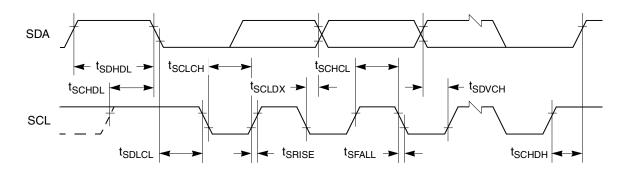
Figure 30. CPM I2C Bus Timing Diagram
