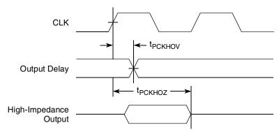
Figure 40. PCI Output AC Timing Measurement Condition
