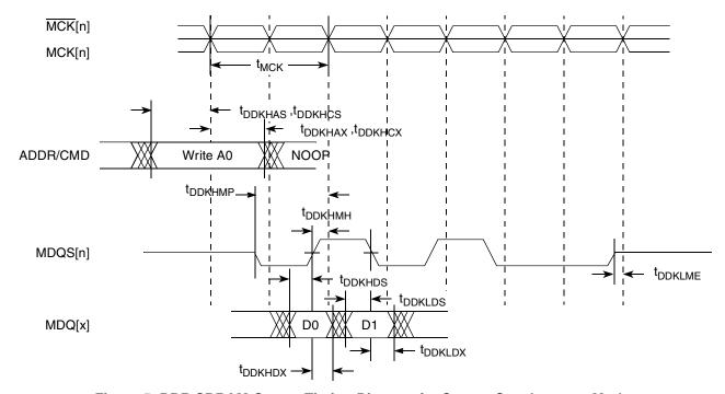
Figure 5. DDR SDRAM Output Timing Diagram for Source Synchronous Mode
