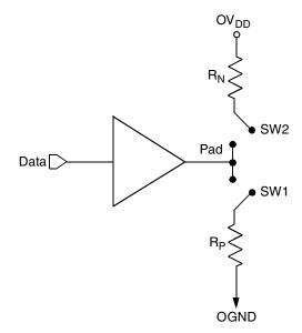
Figure 50. Driver Impedance Measurement
