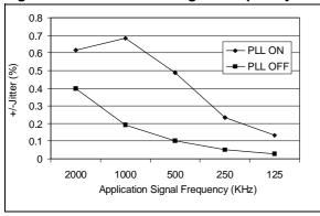
The user must take the PLL jitter into account in the application (for example in serial communication or sampling of high frequency signals). The PLL jitter is a periodic effect, which is integrated over several CPU cycles. Therefore the longer the period of the application signal, the less it will be impacted by the PLL jitter.
