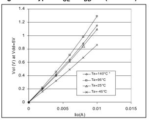
Figure 84. Typical V<sub>OH</sub> at V<sub>DD</sub>=5V
