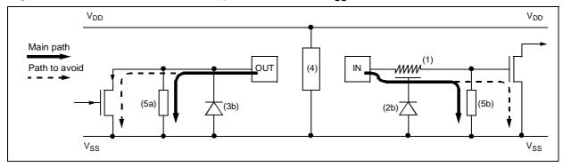
Figure 78. Negative Stress on a True Open Drain Pad vs. V<sub>DD</sub>
