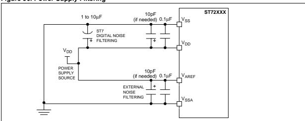
Figure 96. Power Supply Filtering
