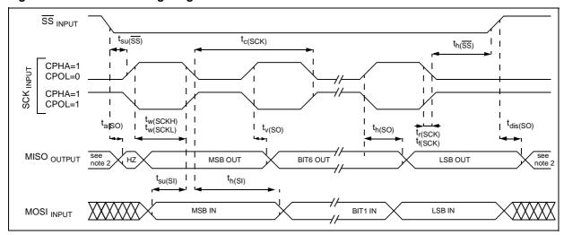
Figure 92. SPI Master Timing Diagram 1)
