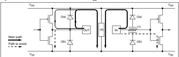
Figure 76. Negative Stress on a Standard Pad vs. V<sub>DD</sub>
