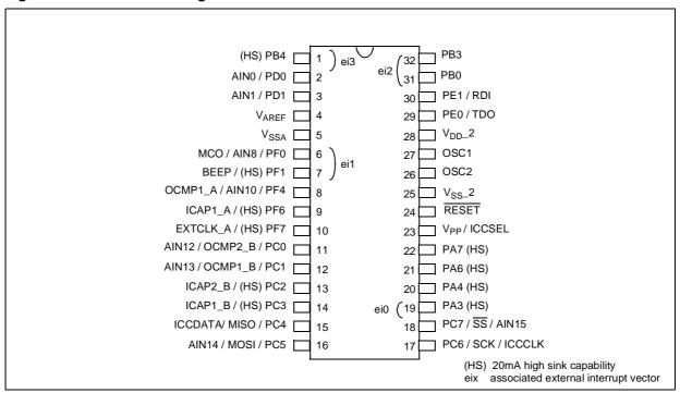
Figure 4. 32-Pin TQFP 7x7 Package Pinout
