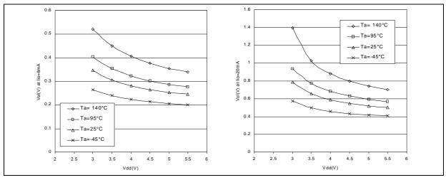
Figure 87. Typical  $V_{DD}$ - $V_{OH}$  vs.  $V_{DD}$
