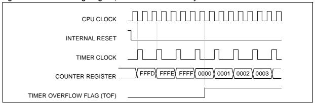
Figure 38. Counter Timing Diagram, internal clock divided by 4
