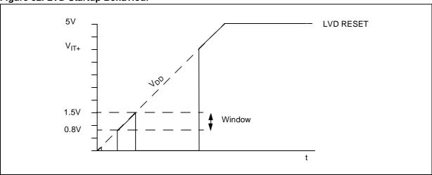
**Note:** When the LVD is enabled, the MCU reaches its authorized operating voltage from a reset state. However, in some devices, the reset state is released when  $V_{DD}$  is approximately between 0.8V and 1.5V. As a consequence, depending on the ramp-up speed, the I/Os may toggle when  $V_{DD}$  is within this window.
