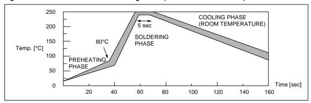
Figure 103. Recommended Reflow Soldering Oven Profile (MID JEDEC)
