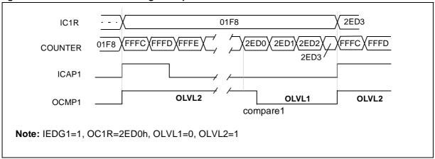
Figure 46. Pulse Width Modulation Mode Timing Example with 2 Output Compare Functions
