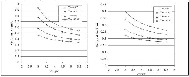
Figure 86. Typical  $V_{OL}$  vs.  $V_{DD}$  (high-sink)
