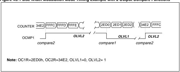
**Note:** On timers with only 1 Output Compare register, a fixed frequency PWM signal can be generated using the output compare and the counter overflow to define the pulse length.
