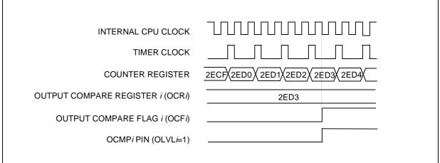
Figure 44. Output Compare Timing Diagram, f<sub>TIMER</sub> =f<sub>CPU</sub>/4
