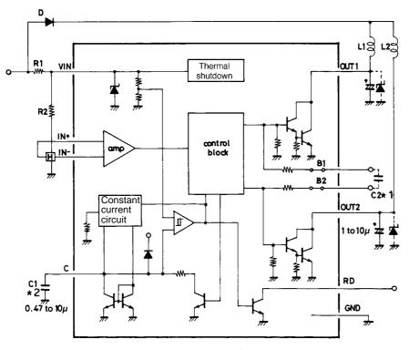
(Note) \*1: Radio noise reduction capacitor: 0.01 to 0.1  $\mu$ F. \*2: Use a less leaky capacitor.
