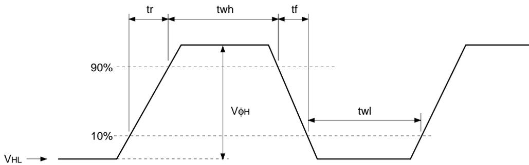
**(4) Reset gate clock waveform**
