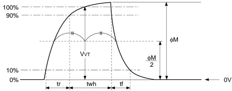
(2) Vertical transfer clock waveform
