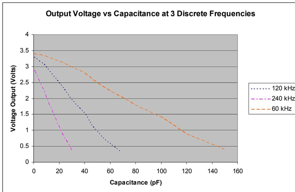
Figure 4. Output Voltage vs. Capacitance at 3 Discrete Frequencies
