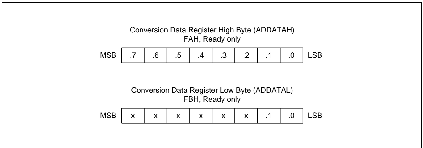
Figure 17-2. A/D Converter Data Register (ADDATAH/L)
