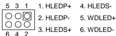
HLEDP: External LED connector for primary IDE channel.
