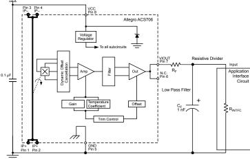
Application 7. Using the FILTER pin provided on the ACS714 eliminates the attenuation effects of the resistor divider between  $R_{\text{F}}$  and  $R_{\text{INTFC}}$ , shown in Application 6.
