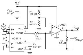
Application 3. This configuration increases gain to 610 mV/A (tested using the ACS714ELC-05A).
