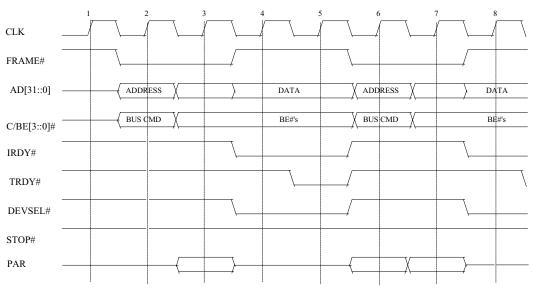
Without contention of TRDY#, DEVSEL#, or STOP#, the IDLE states between transactions are removed. It increase the throughput of the data transaction. If the first transaction is a write cycle and the second transaction access( can be read or write transaction) to the same target , one IDLE cycle can be removed between transactions.
