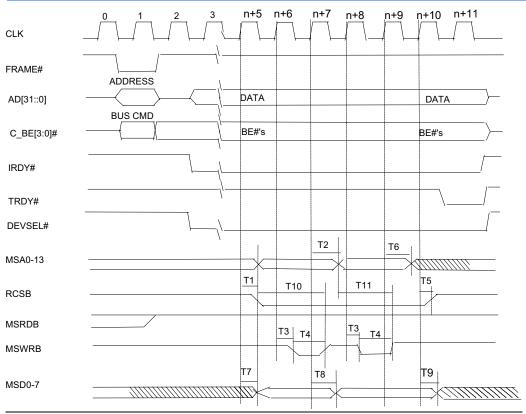
Note: 1) The other timing requirements for PCI signal are as the read transaction timing. 2) n=0,1,2,3,..... when local DMA get the control of the bus, PCI bus will insert wait state.
