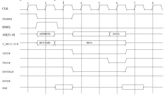
The timing is the same as the figure I/O Read Transaction, except the IDSEL is asserted during the address phase. The transaction access the configuration registers of the device.
