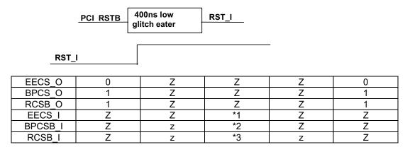
EECS\_O: EECS pin output driver EECS\_I: EECS pin input forcing
